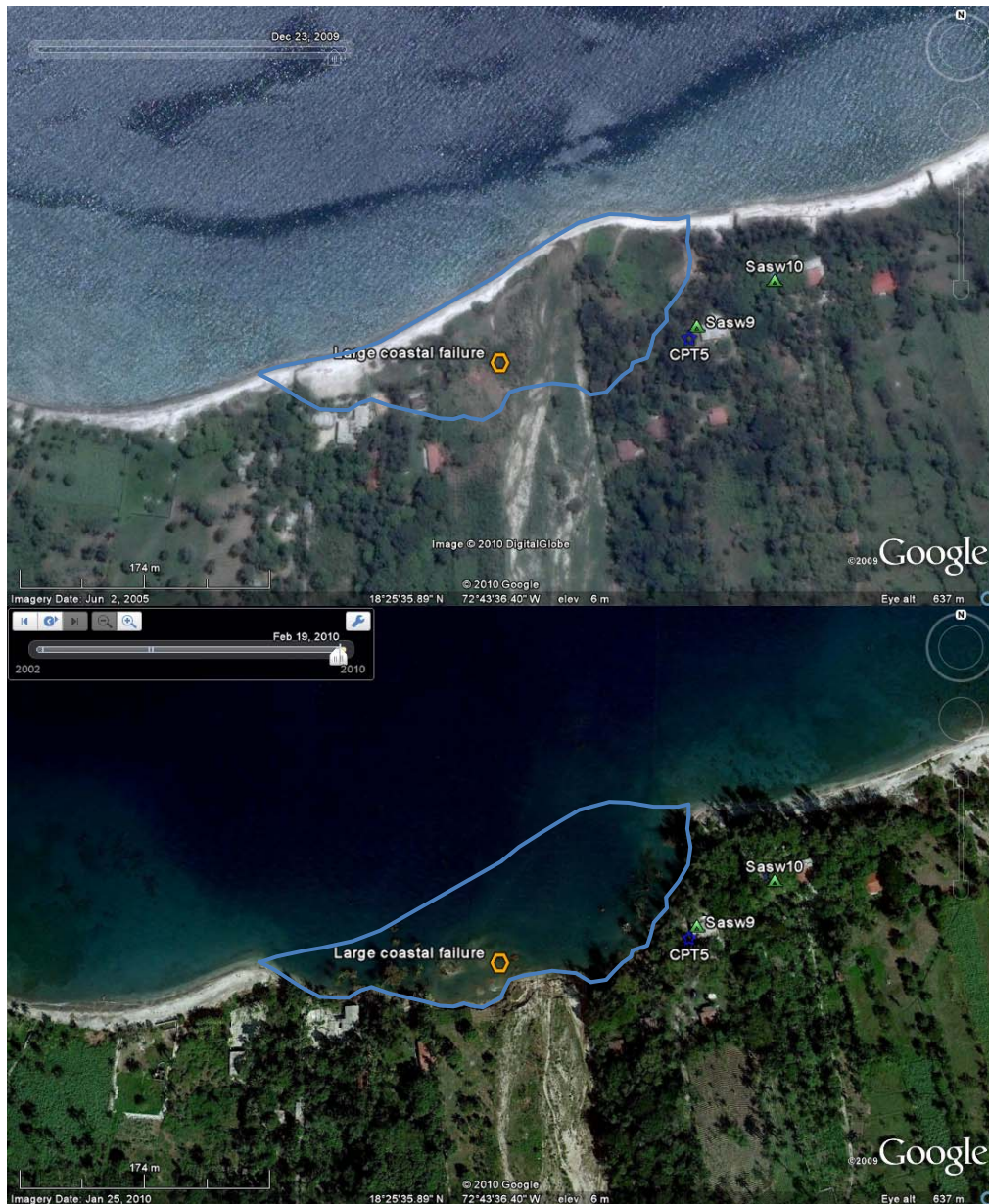
Figure 7.8. Pre- and post-earthquake images of coastline near village of Fouche. Note in the lower, post-earthquake image the significant loss of coast as outlined in blue. SASW-9 and DCPT-6 were performed near several moderate-sized sand blows located near the southeast end of the failure zone, while SASW-10 was performed outside of the failure zone. Imagery courtesy of Google Earth.
