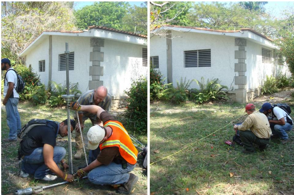
Figure 7.14. DCPT and SASW testing performed at coastal failure site near village of Fouche. Approximate image coordinates: 18^{\circ}25'35.12''\text{N} , 72^{\circ}43'31.61''\text{W} .
