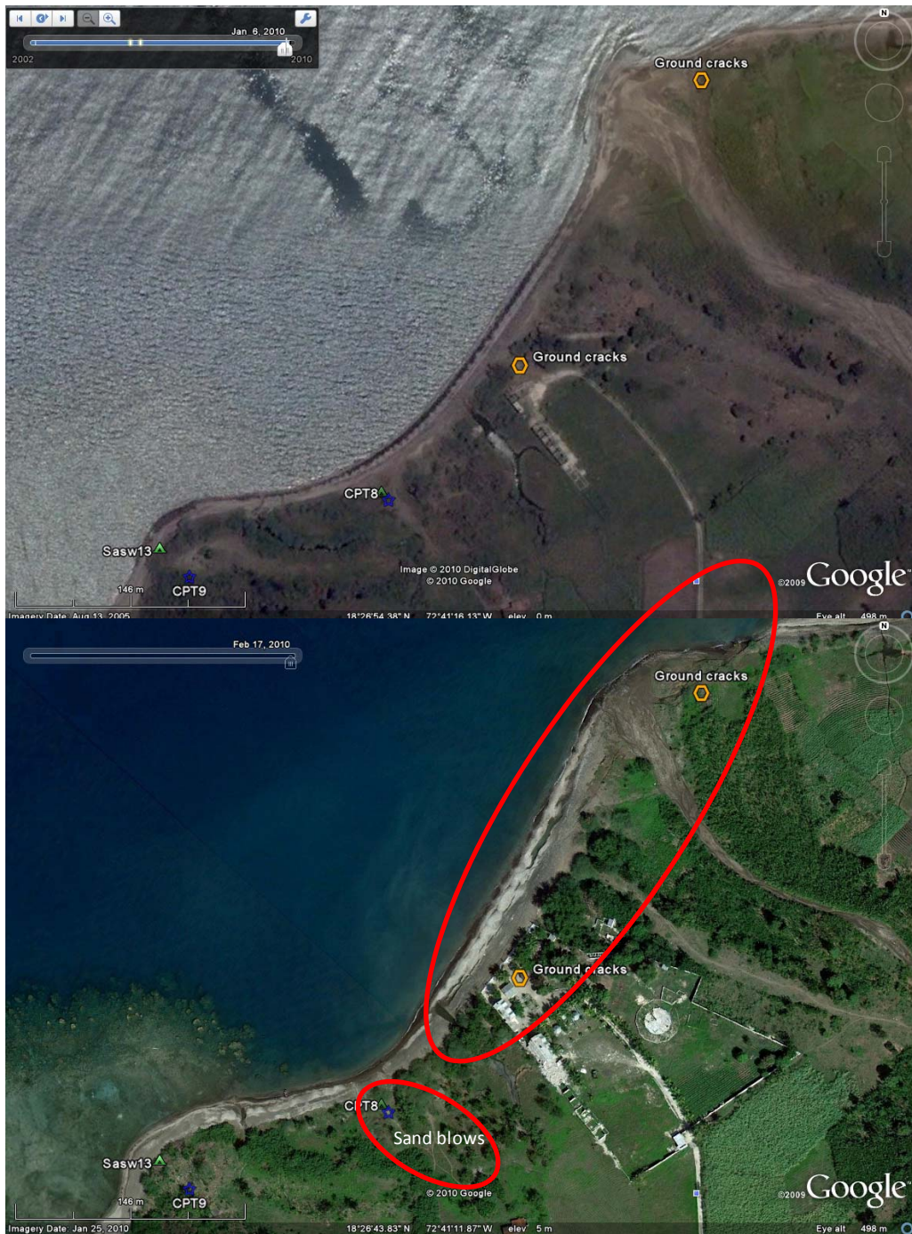
Figure 7.3. Pre- and post-earthquake images of coastline near village of L'Acuil. Note in the lower, post-earthquake image the significant cracking subparallel to the coast and the arcuate slump in the northern end of the failure. SASW and DCPT testing was performed near several large sand blows located near the south end of the failure zone, as well as farther south outside of the failed reach. Imagery courtesy of Google Earth. Approximate center of image at 18^{\circ}26'51.17''\text{N} , 72^{\circ}41'11.06''\text{W} .
